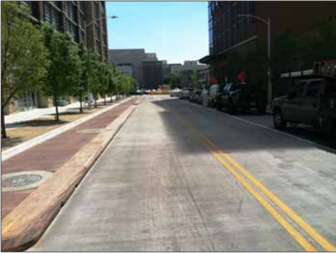
Image 1 - Separated bike lane added because of lane diet
