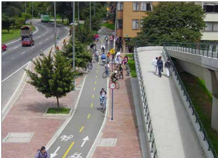
Image 2 - Cycle track separated from main road with wide sidewalks and tree buffer.
