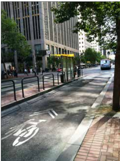
Image 5 - Cycle track separated by raised median with transit uses.
