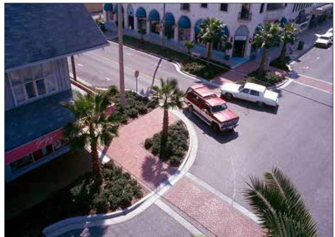
Image 1 - Rounded corner at intersection allows smooth flow of pedestrian activity.
